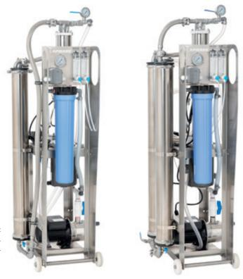
Models shown: One pressure vessel on the left, two pressure vessels on the right. Models shown may differ from your model.
