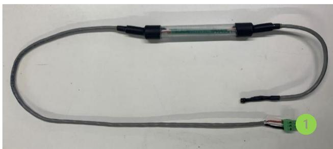
Figure 16 : Internal temperature sensor
