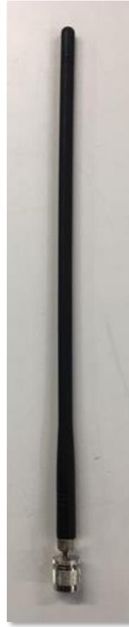
*Figure 29 : Omnidirectional whip antenna and its N connector female socket*
