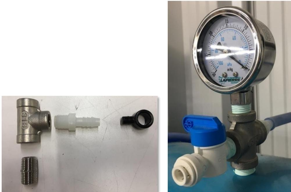
Figure 68 : Connecting the 5/16" (7.94 mm) pipe to the extractor
