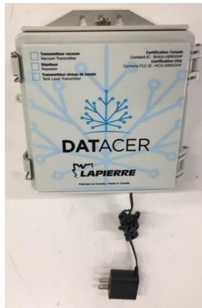
Figure 22 : Connected repeaters without antenna
