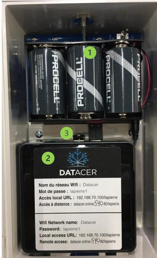
Figure 2 : Interior view of a DATACER™ base
