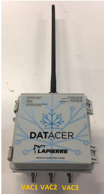
Figure 108 : Significance of the vacuum level measurements on the interface (VAC1, VAC 2 and VAC 3) in relation to the position of the vacuum ports on a transmitter
