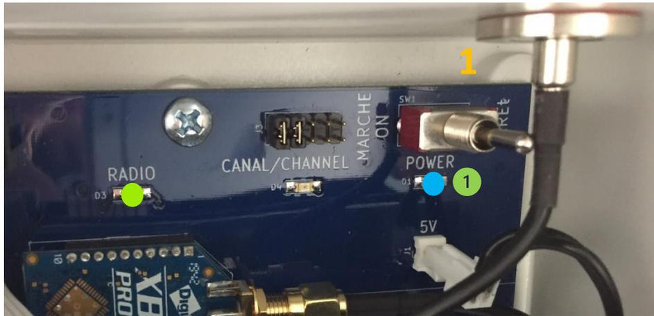
Figure 106 : DATACER™ station radio LED indicator lights
