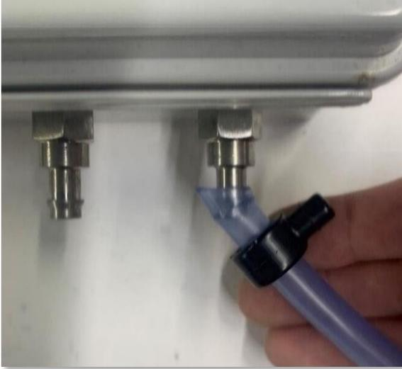
Figure 50 : Bevel cut 5/16" (7.94 mm) pipe for easy installation and removal from the transmitter vacuum port
