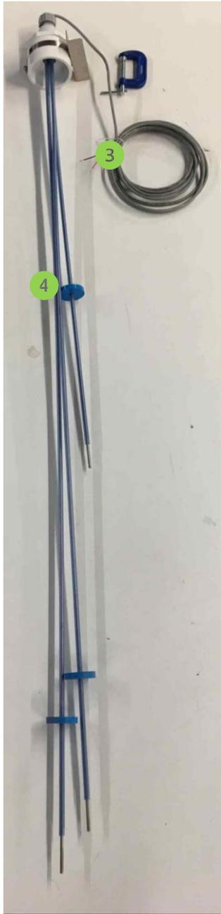
Figure 13 : Water pump control electrodes
