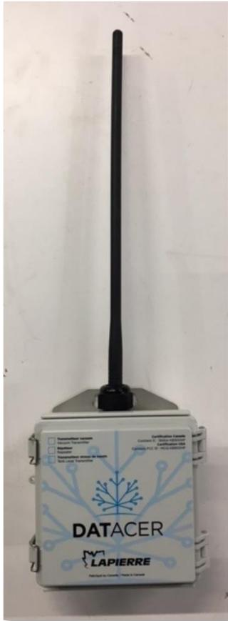
Figure 20 : Battery powered repeater with omnidirectional whip antenna
