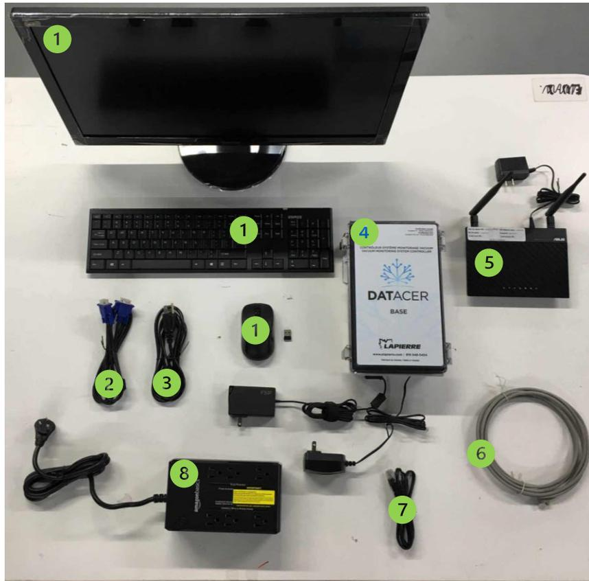
Figure 1 : Components of the DATACER™ base
