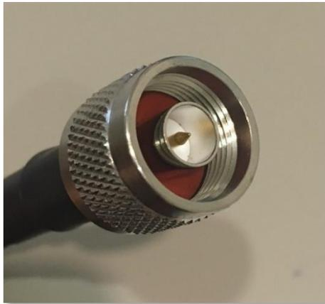
Figure 23 : N Connector male plug socket
