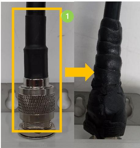
Figure 102 : Transmitter Coax-seal
