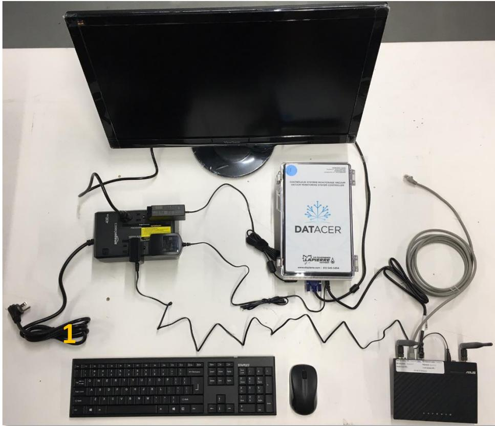
Figure 37 : Connected DATACER™ base
