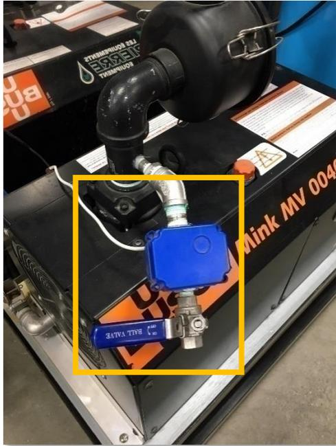
Figure 88 : Air intake valve installed
