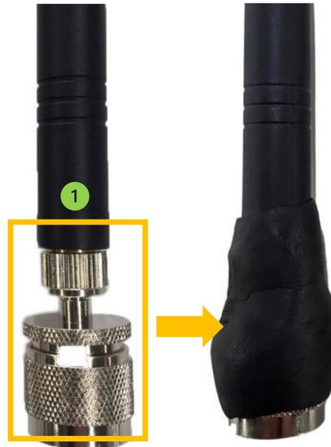
Figure 101 : Antenna Coax-seal option A
