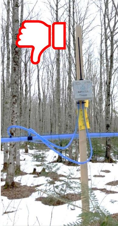
Figure 42 : Vacuum transmitter not properly installed
