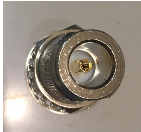
Figure 24 : N Connector female socket
