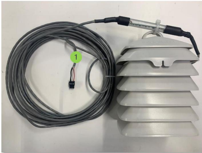
Figure 17 : External temperature sensor
