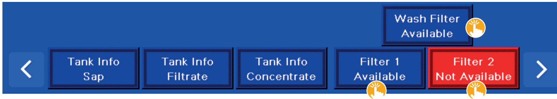
ILLUSTRATION 43 | Tactile key for filter groups 1 and 2 and the Wash filter
