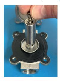
11. CONNECT THE TWO PARTS OF THE ELECTRONIC VALVE | Using the Allen key, screw in the 4 bolts of the electronic valve. Tighten without excess. *Take care to position the valve outlet facing forward, on the same side as the front of the AutoFlo control box.*
