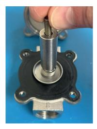
21. ATTACH THE TWO PARTS OF THE ADDITIONAL ELECTRONIC VALVES | Using the Allen key, screw in the 4 bolts of each of the electronic valves. Tighten without excess.
