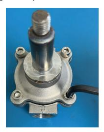
22. PUT THE ACTUATORS BACK IN PLACE | Put the actuators, data plates, and lock washers back in place on each of the valves. The data plates can be reinstalled on any of the valves without distinction. *Take care to position the casing to the left of the valve outlet.* Then, tighten each of the cap nuts without excess using the 14 mm key.
