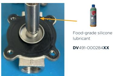
10. INSERT THE SPRING INTO THE CENTRAL ROD OF THE VALVE
