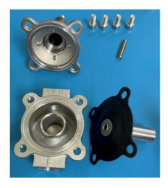
18. PUT THE MEMBRANES BACK IN PLACE ON THE BASES OF THE ELECTRONIC VALVES | At this stage, pay attention to the following indication: the position of the valve outlets (indicated by an arrow grooved directly into the base of the valve outlet) vs. those of the small holes in the membranes.
