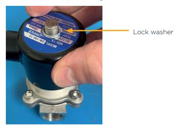
16. SEPARATE THE TWO PARTS OF THE ADDITIONAL ELECTRONIC VALVES | Using the Allen key, unscrew the 4 bolts of the electronic valves (1). Then, **carefully** *open the valve* (2), since some parts, with a sudden movement, could detach and fall. Special attention should be paid to the spring inserted freely into the central rod of the valve. Finally, gently separate the central rod and its membrane from the base of the electronic valve.
