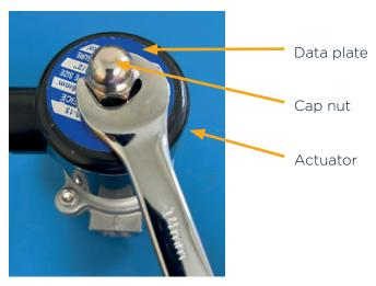
15. REMOVE THE ACTUATORS | Gently lift and remove the actuators.
