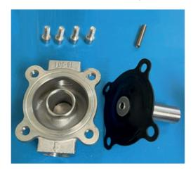
7. CLEAN THE UPPER PART OF THE VALVE | The upper part of the electronic valve attached to the AutoFlo control box is cleaned using a twisted cloth soaked in hot water and a pipe cleaner-type brush (*Illustration 12*). Note that the cavity in the upper part which accommodates the central valve rod and the spring is 14 mm (0.55 in.) in diameter. This measurement could be useful in choosing your pipe cleaner.
