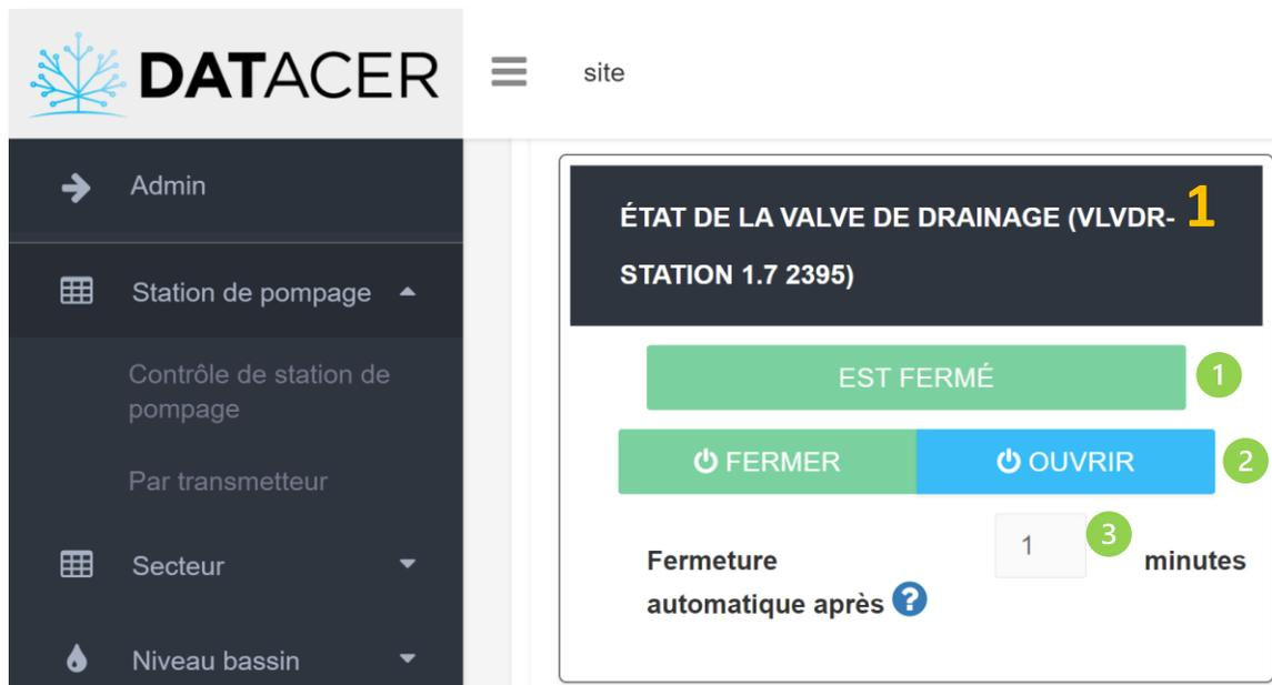
The screenshot shows the DATACER interface for a drainage valve. The title is 'ÉTAT DE LA VALVE DE DRAINAGE (VLVDR-1 STATION 1.7 2395)'. Below the title, there is a green bar indicating the valve is 'EST FERMÉ' (1). Below this, there are two buttons: a green 'FERMER' button and a blue 'OUVRIR' button (2). At the bottom, there is a timer for 'Fermeture automatique après ?' (3) set to 1 minute.
