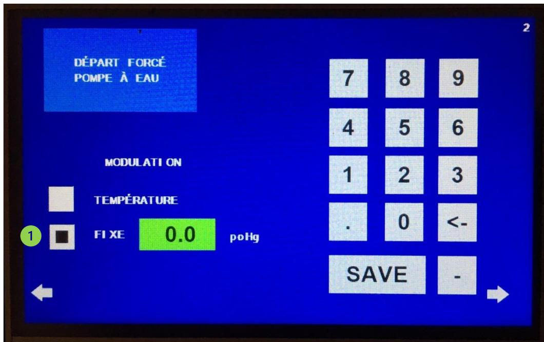
The screenshot shows the DATACER station interface. At the top left, a blue box displays 'DÉPART FORCÉ POMPE À EAU'. Below it, the 'MODULATION' section shows 'TEMPÉRATURE' selected and 'FIXE' selected (highlighted with a yellow '1'). The 'FIXE' value is '0.0 poHg' (highlighted with a yellow '2'). A numeric keypad is on the right, and a 'SAVE' button is at the bottom.
