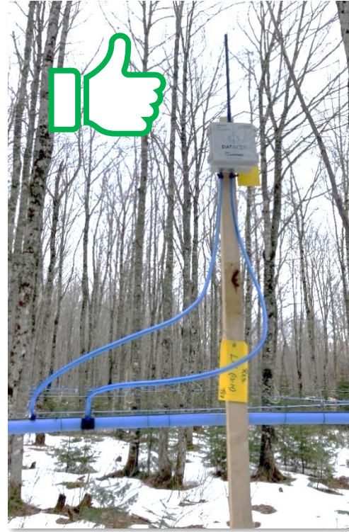
Figure 48 : Vacuum transmitter properly installed
