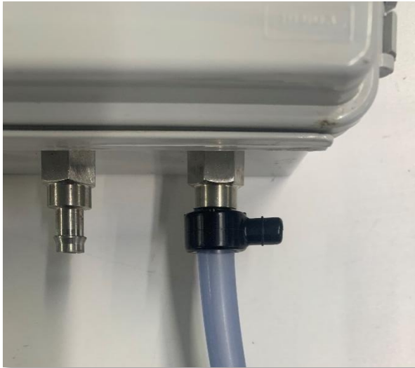
Figure 55 : Bevel cut 5/16" (7.94 mm) pipe for easy installation and removal from the transmitter vacuum port
