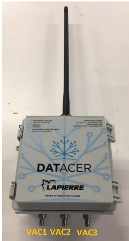
Figure 131 : Significance of the vacuum level measurements on the interface (VAC1, VAC 2 and VAC 3) in relation to the position of the vacuum ports on a transmitter
