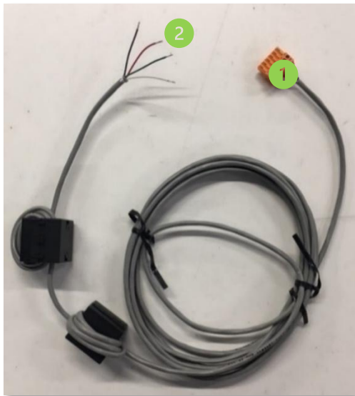
Figure 10 : Connection for start/stop and speed variation of a vacuum pump with drive
