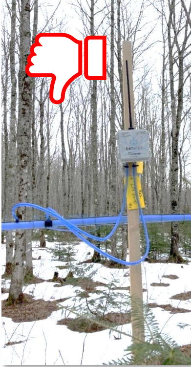
Figure 47 : Vacuum transmitter not properly installed
