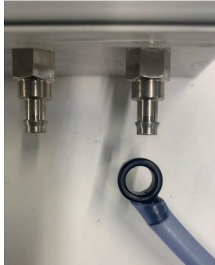
Figure 55 : Bevel cut 5/16" (7.94 mm) pipe for easy installation and removal from the transmitter vacuum port
