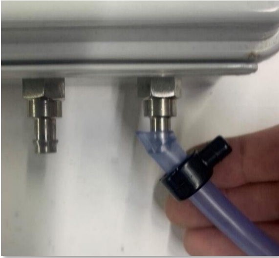
Figure 55 : Bevel cut 5/16" (7.94 mm) pipe for easy installation and removal from the transmitter vacuum port
